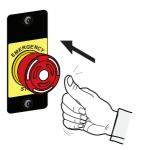
• To reset the door to normal operation - release the emergency stop button by rotating it in the direction of the arrows and press reset button.
